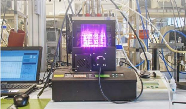
Growing cyanobacterial cell factories under well-controlled photoautotrophic conditions.
