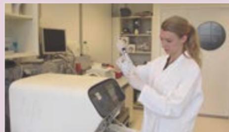
The Ion Proton is being prepared for a sequencing run.
